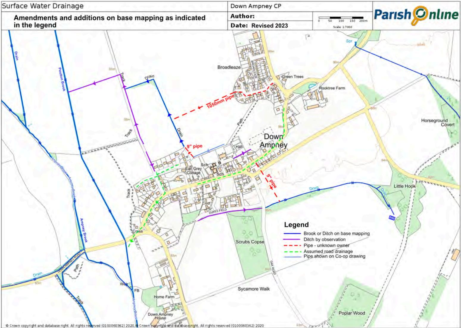
Figure 5.4 Surface Water Drainage Detail
