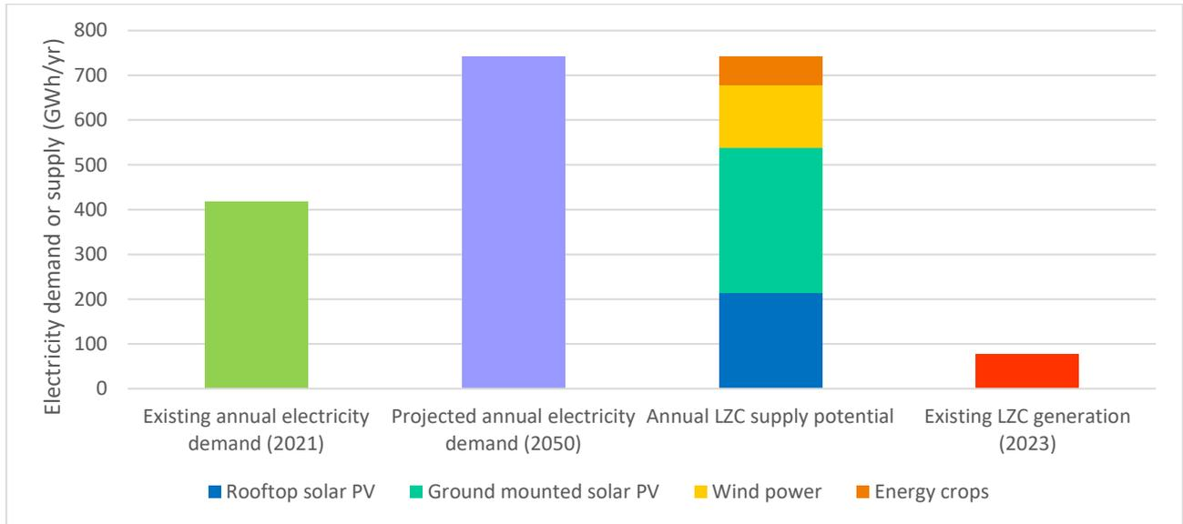
Figure 11 shows scenario 4, which diverges from FES assumptions and conforms to the target set in the balanced pathway of the 6<sup>th</sup> Carbon Budget report. This states that 80% of electricity demand should be met by variable renewables by 2050. This scenario uses a mix of the four energy sources to meet 2050 projected annual demand: 225.8 MW of rooftop solar, 300.5 MW of ground mounted solar, 47.5 MW of wind and 10 MW of energy crops.
