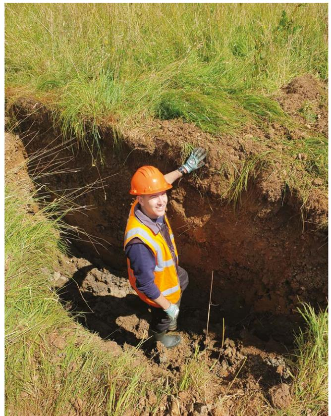
**Fig. 4.** NCP Project Officer assessing substrate in a test pit.
